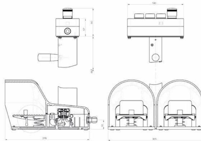
Available double foot switch IP7027 with PQ04 station 4 holes with EN ISO 13850 emergency stop.
