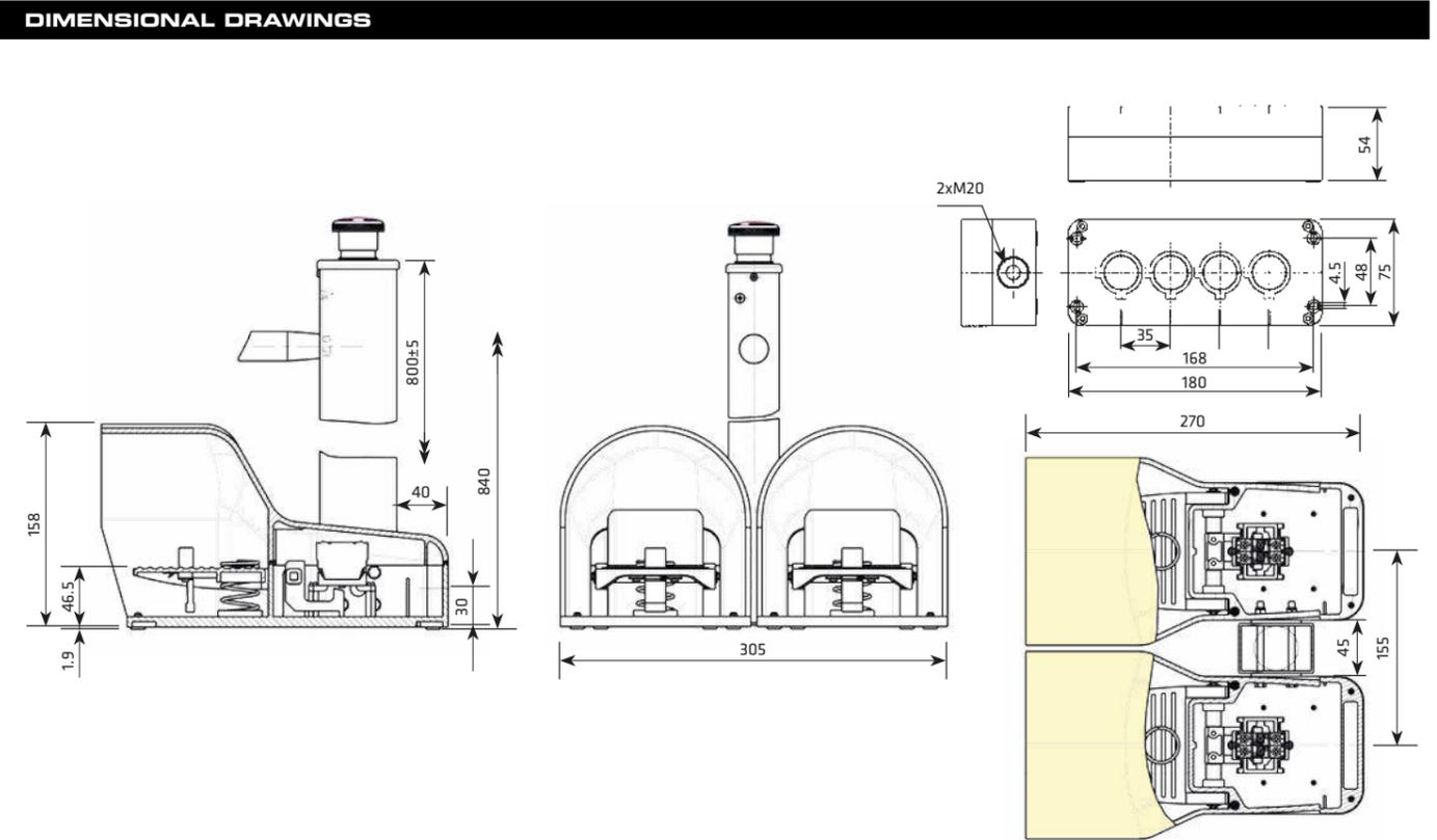
Double foot switches thermoplastic type with EN ISO 13850.
